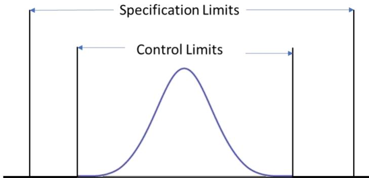
ACME's production line is capable, meaning that it produces a very low defect rate when it is running well. The common cause variation present in this process is bounded by the control limits. When the process is centered, it will make almost no parts out of spec. In Figure XX we see that the control limits are tighter than the specification limits. This means we will almost never get out of spec parts from this process when only common cause variation is present.
