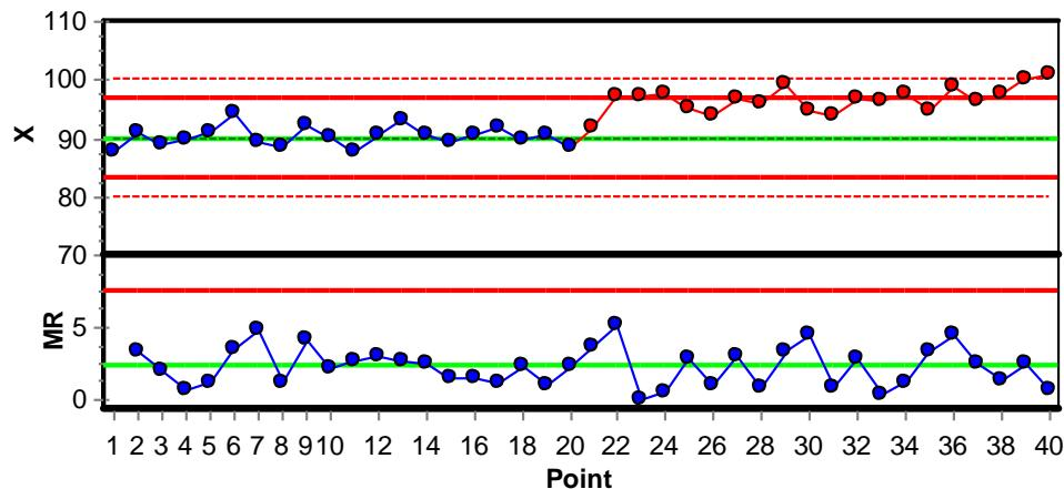
The above example highlights what happens when an abrupt change is made to the process. However, if the shift occurs over time, for example, due to wear, the use of SPC run rules would likely detect the increase prior to the process making any parts out of specification. This allows the operator to stop the process and address the root cause without having to hold and inspect any parts.
