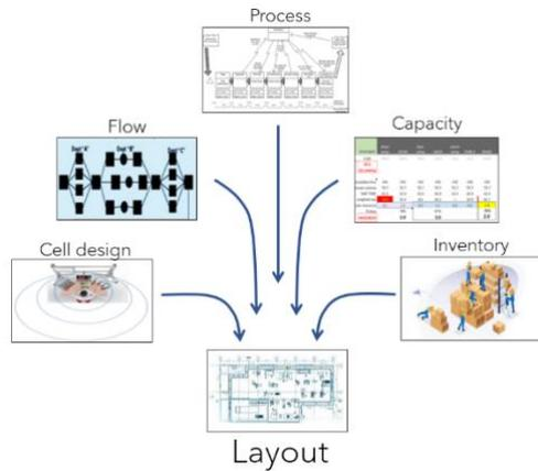
The goal of this final component is to incorporate all the previous discoveries and to lay out the facility to optimize the relationships of areas that need to be close to each other and minimize the negative interactions in support of high quality and efficient operations. This is the time to consider safety, communications, utility availability, floor strength, access to windows, doors and docks, air quality, and noise.
